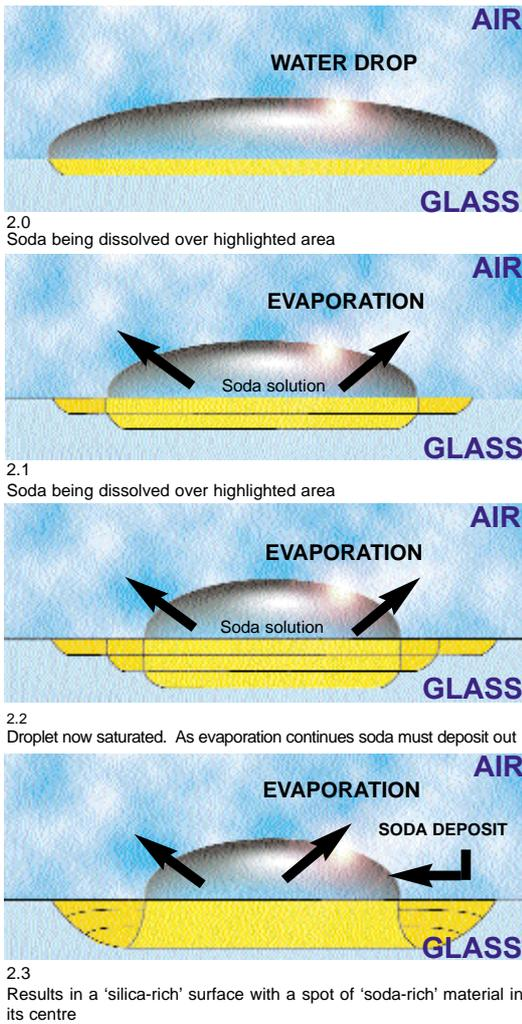
**Figure 2. Evaporation of a water droplet on new glass surface**
